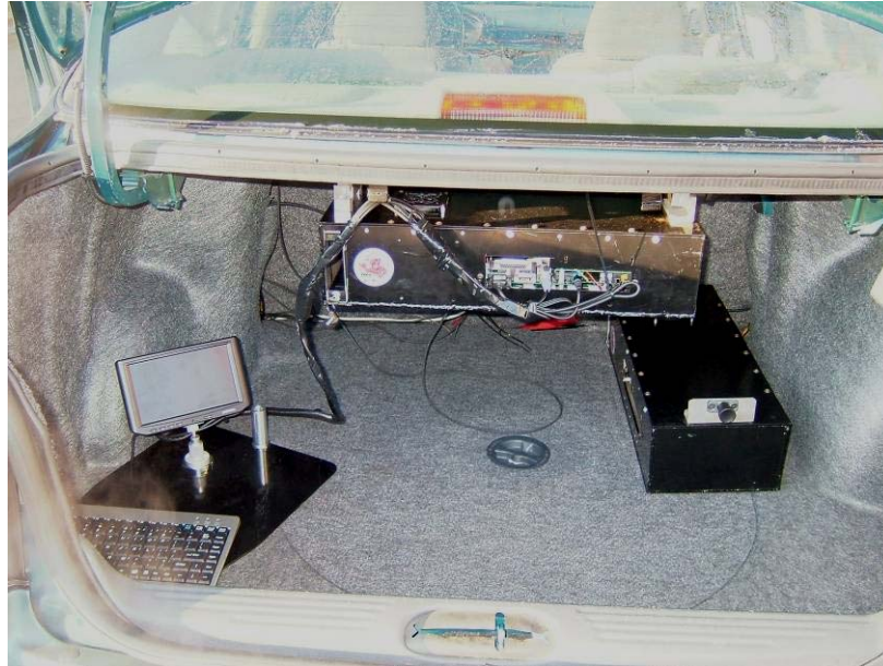
Figure 12. Data Acquisition System Located in Trunk of Vehicle.
