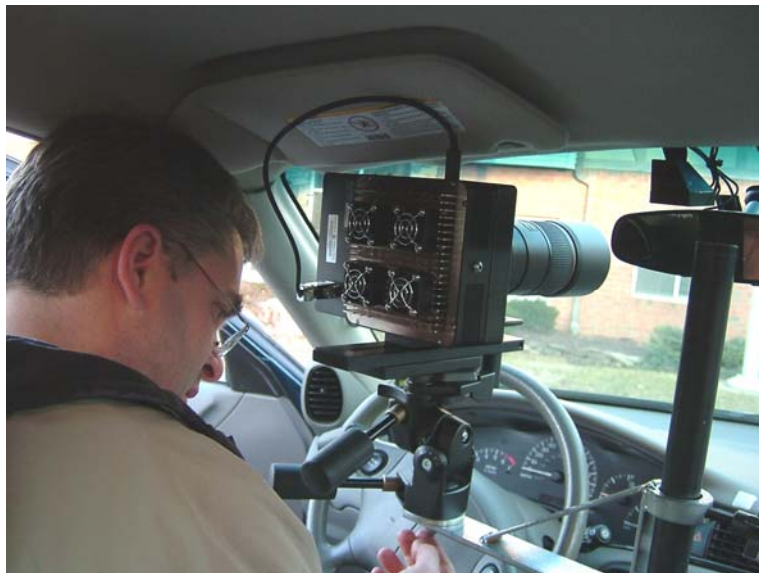
Figure 35. Radiant Imaging CCD Photometer in Position for Measurements, with Experimenter Making Final Adjustments.
