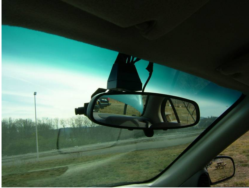
Figure 10. Driver Face Camera Mounted Above Rear View Mirror.
